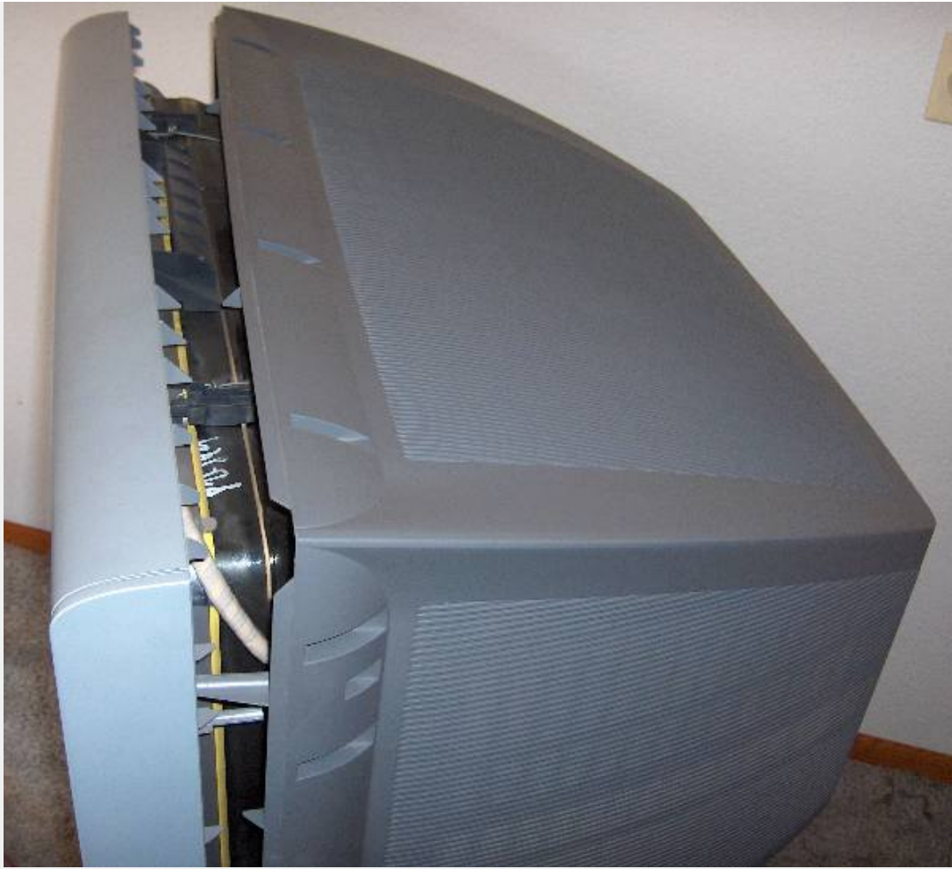
Fig 1. After removing about a 17 screws, the rear shell can be slipped off.
